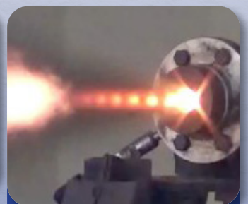
Static Fire Test of Solid Propellant
