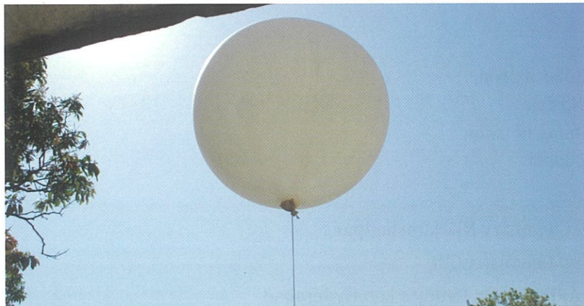
Radiosonde observations for upper boundary layer
