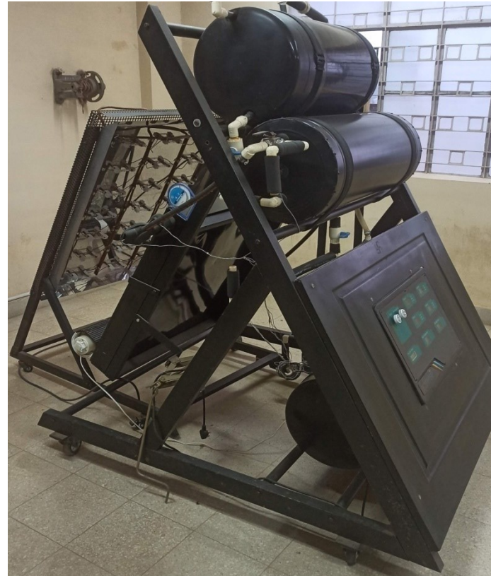
Solar water Heating System (Thermo Syphon type)
