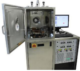
Multi-target E-beam evaporation system
