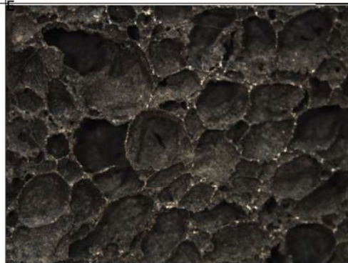
Optical microscopy image of aluminum foam at 12x magnification. Such Aluminium foam has properties, which make them suitable for structural, energy absorption and acoustic applications.
