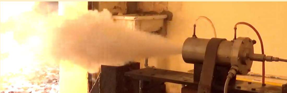
Kerosene-Gaseous Oxygen (Thrust = 100 N)
