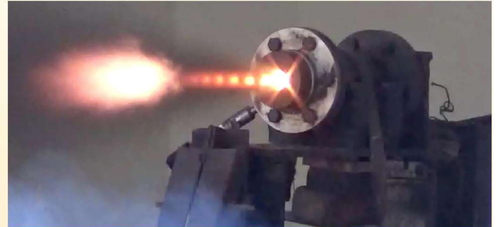
Exhaust from a Static Fire Test of Solid Propellant
