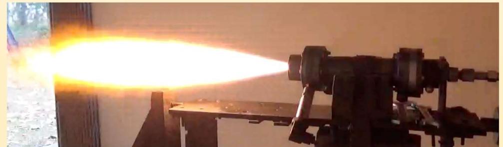
Wax-Gaseous Oxygen Hybrid Propellant (Thrust = 50 N at 7 bar)
