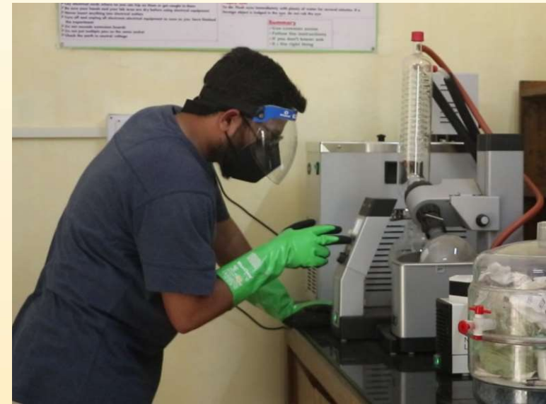
Concentration of Hydrogen peroxide using Rotary Evaporator
