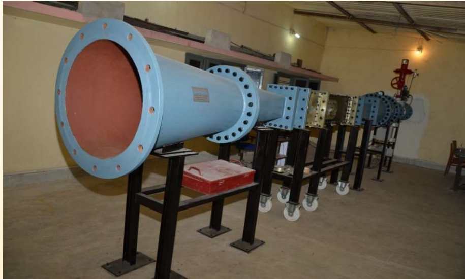
Supersonic Wind Tunnel (100mm x 150mm, Mach 1.5 to 3.5)
