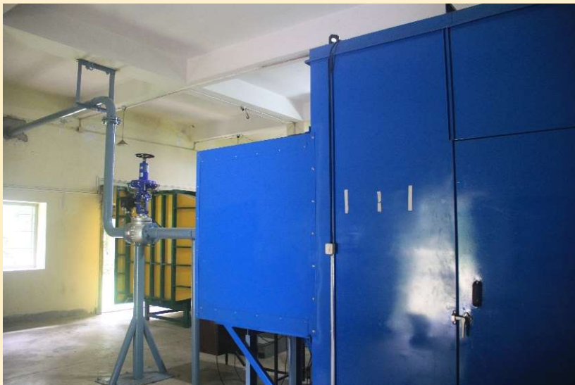
Supersonic Wind Tunnel (100mm x 150mm, Mach 1.5 to 3.5)
