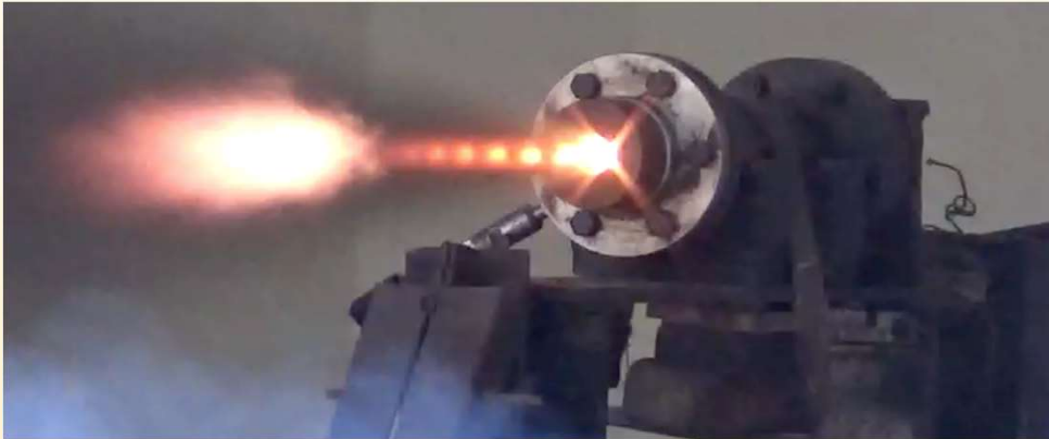
PVC-AP Composite Solid Propellant (Thrust = 750 N at 60 bar)
