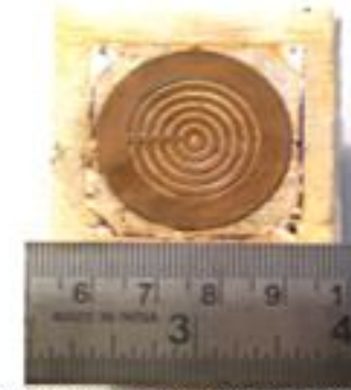
Figure 14: Fabricated Layout of BW reconfigurable Circular ring patch antenna. Resonance frequency 3.5 GHz and BW 200 MHz.
