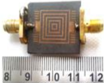
Figure 16: Fabricated Layout of BW reconfigurable Square ring Bandpass Filter. Resonance frequency 3.5 GHz
