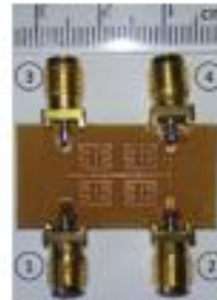
Figure 10: A compact parallel coupled meander lines shaped CRLH-TL based symmetric quasi-0 dB coupler
