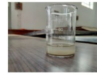
Fig. III (c): Powder immersed in isopropanol for hydration stoppage (TGA, XRD)
