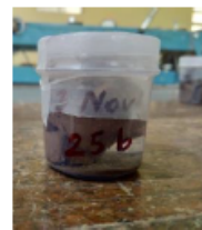
Fig. II (b): Cement paste cured inside plastic vessel sealed with Parafilm
