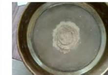
Fig. III (b): Powder being sieved through 63µ sieve
