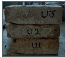
Fig. I (a): Underburnt bricks as obtained from the kiln
