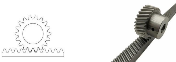
Fig-2: Picture showing rack and pinion for converting the rotary motion of the focusing knobs to translatory motion of the inner tube of the telescope or the collimator.
