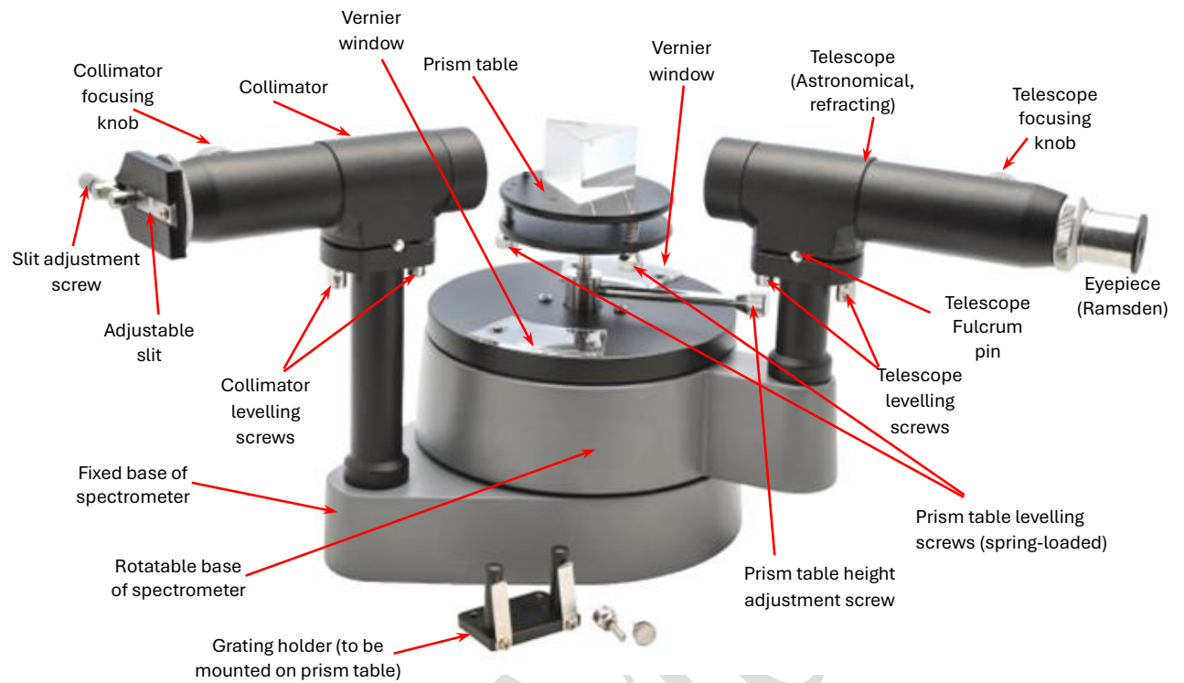
Fig-1A: Picture showing a student grade laboratory spectrometer, its components, adjustment knobs and screws.
