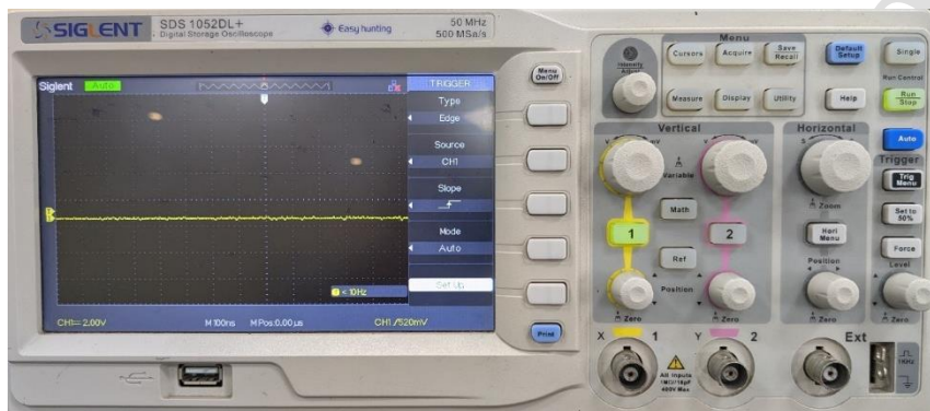
Fig-2. Actual image of the front panel of a digital storage oscilloscope (CRO)
