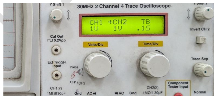
Fig-1. Actual image of a relevant portion of the front panel of a cathode ray oscilloscope (CRO)
