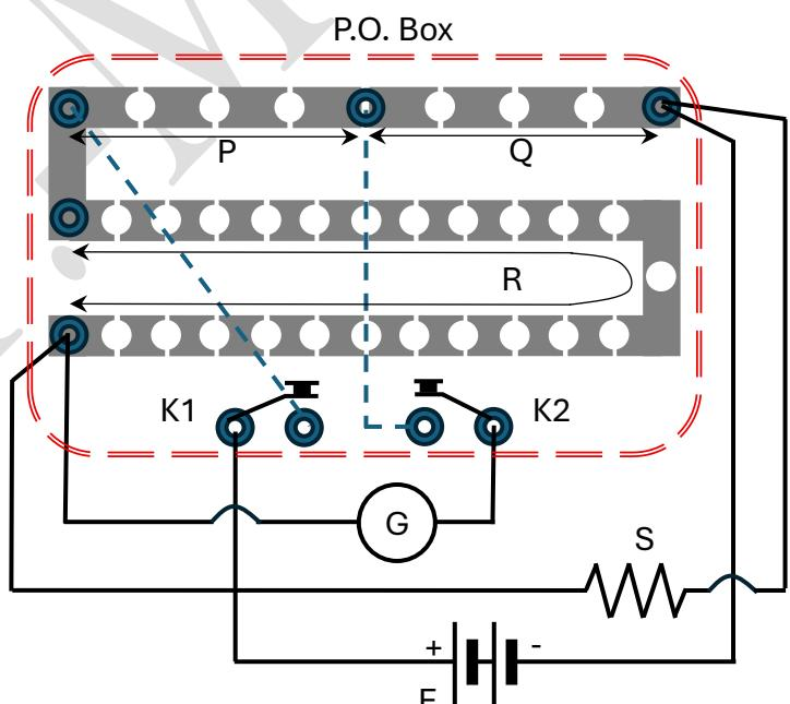
Fig-1. Wheatstone bridge circuit for the determination of value of a resistance.
