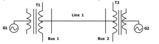
Choose 25kV as the base voltage at the generator 1 side, and 200MVA as the base MVA base. Draw the impedance diagram.
