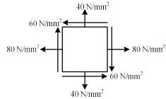
Q.4(b) Draw the Mohr's circle for the stress condition given in Q.4(a). Using the Mohr's circle [5] 3 determines the normal and shear stresses on an oblique plane making an angle  $45^{\circ}$  anticlockwise with the x-plane.
