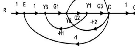
Find C(s)/R(s) of given line diagram using mason's gain formula
