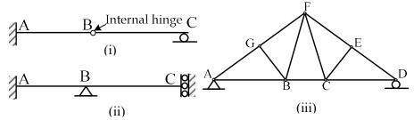
Q.2(a) Consider the cantilever beam shown in the following figure where the free end of the beam (end C) is propped with a roller support, and there is an intermediate hinge at B. Span AD is subjected to udl of intensity 5 kN/m and span DB is subjected to uvl varying for 5 kN/m to 10 KN/m as shown in the figure. A clockwise couple of 15 kN-m acts at end C. Find the support reactions at A, B and C.
