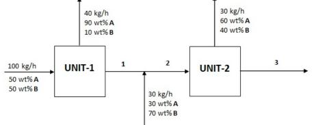
(i) Perform the degree-of-freedom analysis of the following: overall system, Unit 1, mixing point, and Unit 2.
