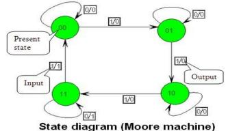
4. Outline a VHDL/Verilog model and write RTL code for a Mealy machine with the following state transition diagram. Simulate/compile the same using the Xilinx development software (Xilinx ISE 8.1i./10.1i) and find errors, if any. Test for its operation and analyse the results.
