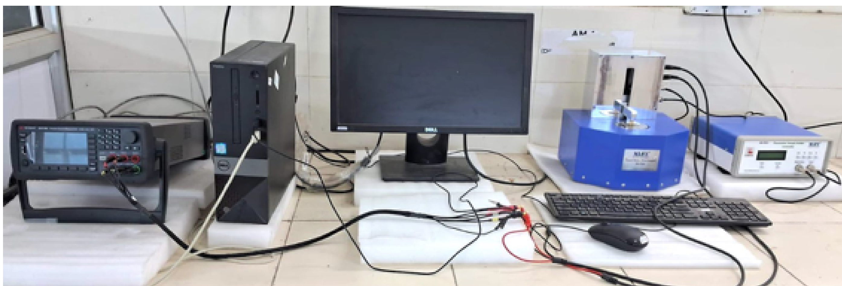
SOURCE METER (USB/GPIB Interface) with Kelvin Probe Set, Piezo Sample Holder
