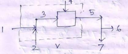
one can write independent material balance equations of two or more equations of combinations of two or more units simultaneously, as indicated by (V, vi and to boxes. (dotted).
