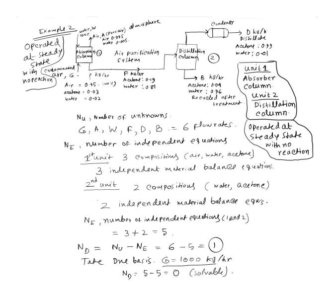
Material balance for multiple units with recycle, purge, and by pass streams
