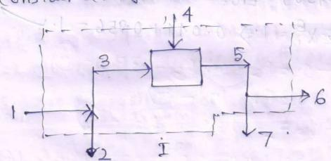
The dotted box reprents the overall process (I) where imput streams are 1, 2, 4, and output streams are 6 47,
